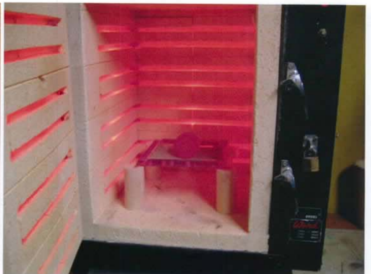
Fig.2: Stainless steel sample at 800 degrees Celsius.
