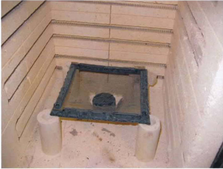
Fig 7: Stainless steel sample cool after failure.
