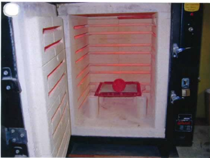
Fig.3: Stainless steel sample at 850 degrees Celsius.
