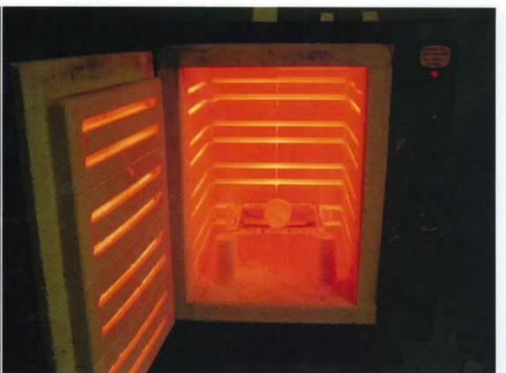
Fig.6: Stainless steel sample at 1000 degrees Celsius.
