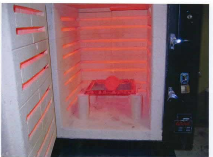
Fig.4: Stainless steel sample at 900 degrees Celsius.
