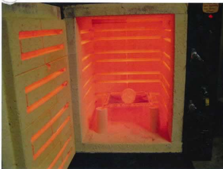
Fig.5: Stainless steel sample at 950 degrees Celsius.
